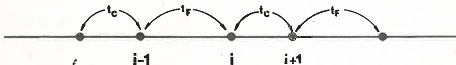
Fig. 1. Distorted atomic chain with one electron per atom. The electron hopping integrals between neighbour sites are noted
