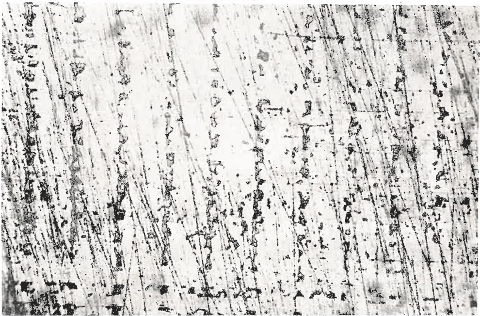
Fig. 2b. Etching figures of section through plane (001)
