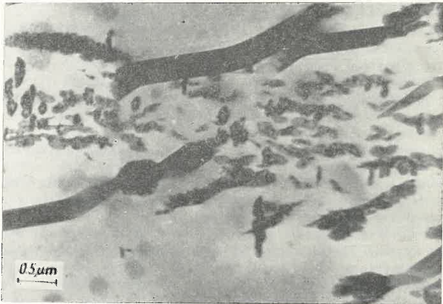
Fig. 2. The microstructures of iron samples aged for 0.5 h at 528 K, and then additionally for 3 hrs at 383 K
