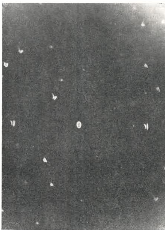
Fig. 10. Lauegram taken on a crystal with precipitates
