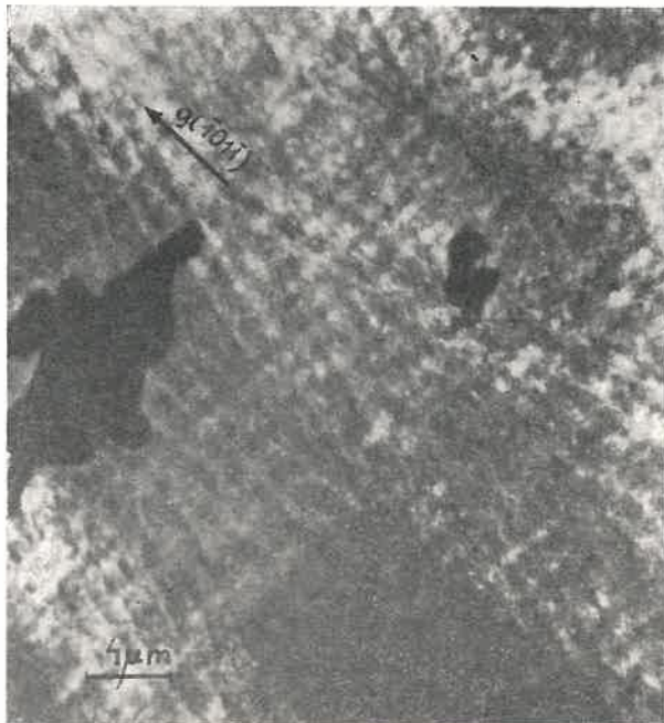
Fig. 4. Two different systems of excess zinc precipitates
