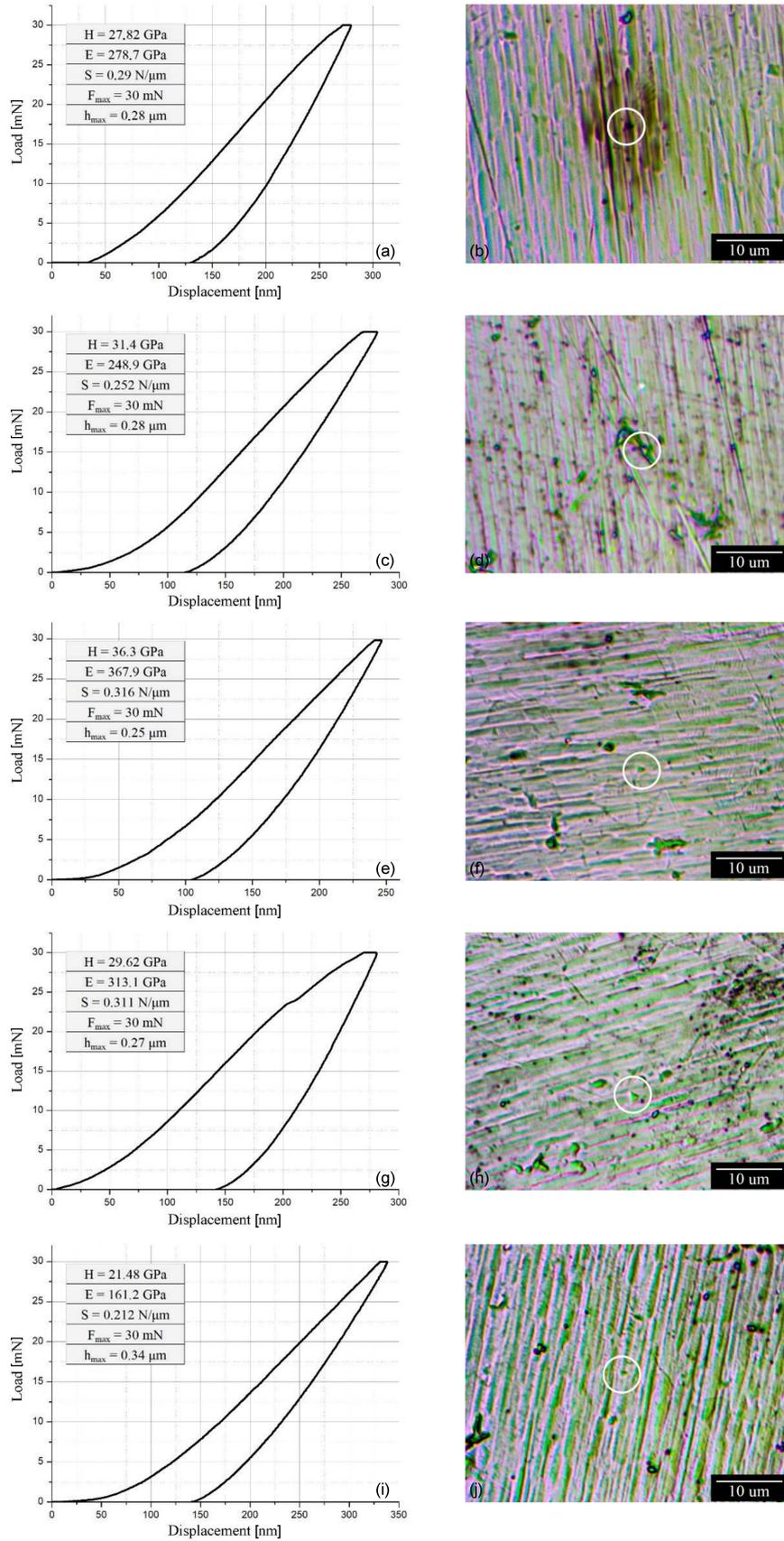
Fig. 3. Load-unload curves (a, c, e, g, i) and micrographs of indenter prints (b, d, f, h, j) from a TiAlN coating irradiated with Ar<sup>+</sup> ions with various fluences: (a, b) — as-deposited; (c, d) —  $2.5 \times 10^{16}$  ions/cm<sup>2</sup>; (e, f) —  $5 \times 10^{16}$  ions/cm<sup>2</sup>; (g, h) —  $1 \times 10^{17}$  ions/cm<sup>2</sup>; (i, j) —  $2 \times 10^{17}$  ions/cm<sup>2</sup>.
