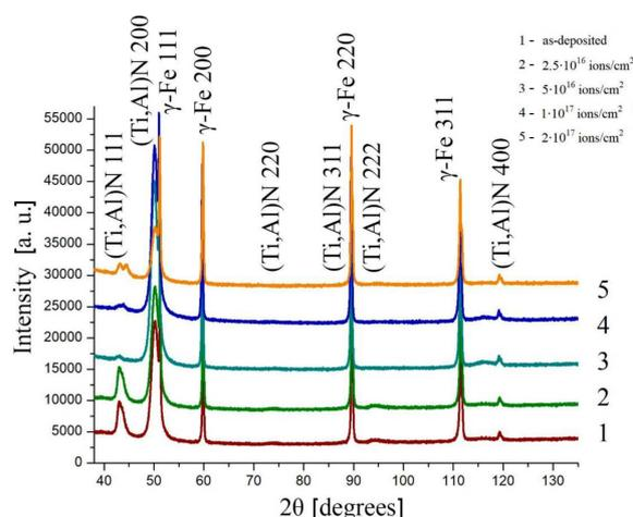
Fig. 2. X-ray diffractograms from TiAlN coatings in the initial state and irradiated by 200 keV  $\text{Ar}^+$  ions at a temperature of 480 °C with various fluences.
