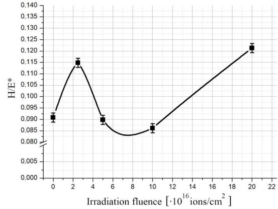
Fig. 5. Dependence of the index of impact strength ( $H/E^*$ ) of the TiAlN coating on the fluence of irradiation with 200 keV Ar $^+$  ions at a temperature of 480 °C.
