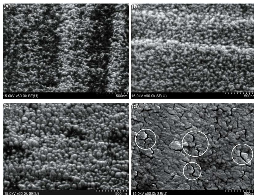
Fig. 1. SEM micrographs of surface of TiAlN coatings irradiated by 200 keV  $\text{Ar}^+$  ions at 480°C with fluences: (a)  $2.5 \times 10^{16}$  ions/cm<sup>2</sup>; (b)  $5 \times 10^{16}$  ions/cm<sup>2</sup>; (c)  $1 \times 10^{17}$  ions/cm<sup>2</sup>; (d)  $2 \times 10^{17}$  ions/cm<sup>2</sup>.
