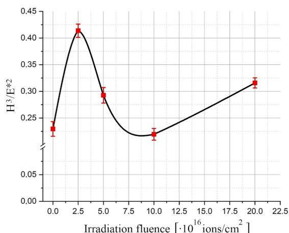
Fig. 6. Dependence of the plastic deformation index ( $H^3/E^{*2}$ ) of the TiAlN coating on the fluence of irradiation with 200 keV  $\text{Ar}^+$  ions at a temperature of 480°C.
