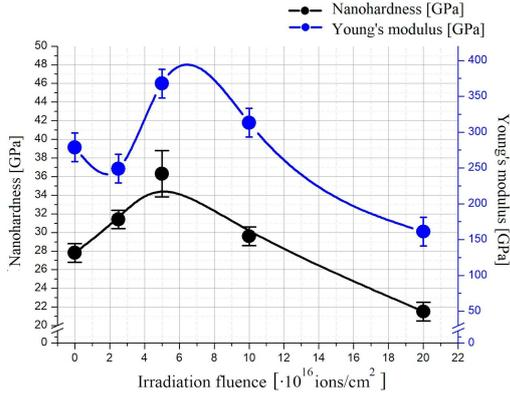
Fig. 4. Dependence of nanohardness and Young's modulus of TiAlN coatings on the fluence of irradiation with 200 keV Ar $^+$  ions at a temperature of 480°C.
