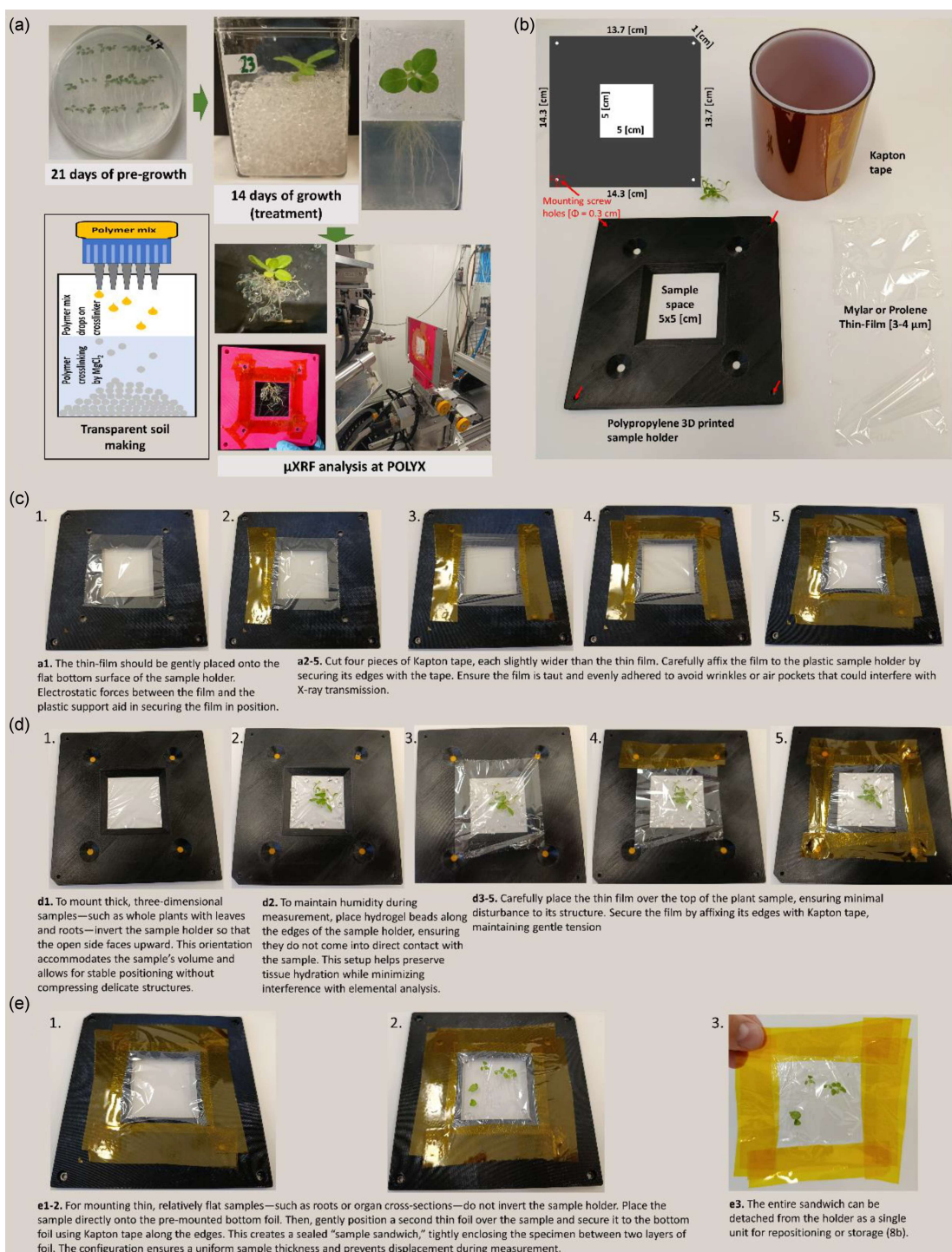
Fig. 1. Experimental design for \mu XRF analysis of plant samples. (a) Schematic representation of the plant growth protocol leading up to \mu XRF analysis. (b) Material used for sample preparation, including the design of the custom sample holder with adjustable thickness; here, a 0.5 cm thickness was used. (c) Mounting procedure for basic support film onto the sample holder. (d) Configuration for mounting thick 3D samples, such as whole plants with leaves and roots. (e) Mounting approach for thin, flat samples, such as roots or organ cross-sections, using a dual-film “sandwich” technique.
