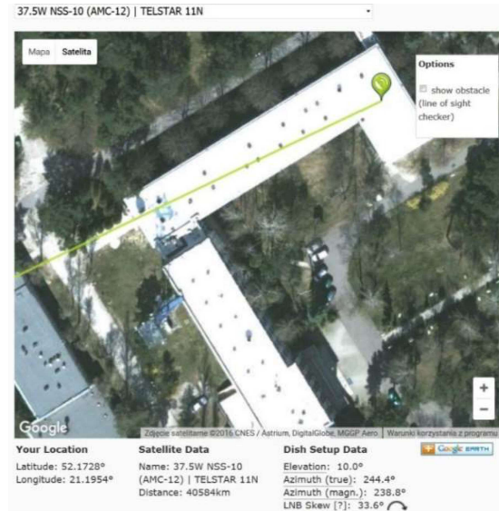
Fig. 3. Direction of satellite dish for TWSTFT in NIT's location for the T11N satellite (see [10]).
