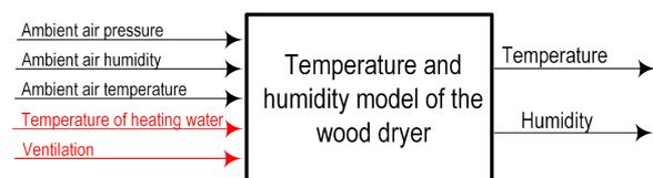
Fig. 1. Block diagram of the temperature and humidity model of the wood dryer.
