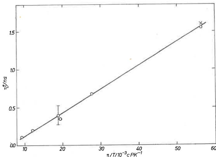
Fig. 3. Dependence of  $\tau_D^*$  on  $\eta/T$  for acridine orange. Excitation at 450 nm; measurement at 550 nm.  $\circ$  —  $1.1 \times 10^{-3}$  mole/l in a glycerol-water mixture 50:50,  $\times$  —  $6.0 \times 10^{-5}$  mole/l in undecanol
