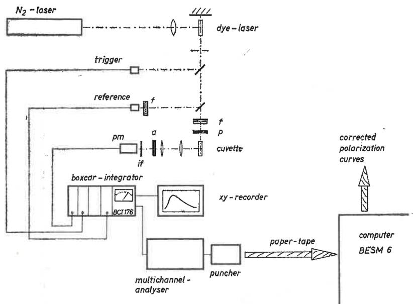
Fig. 1. Experimental set-up of laser spectrofluorimeter (for description see text)
