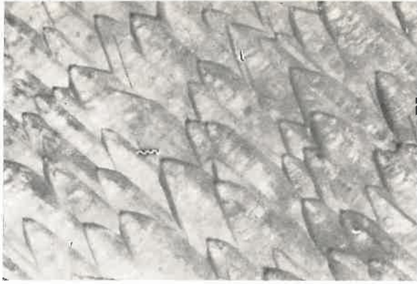
Fig. 6. The etch figures on the cross section of crystals perpendicular to the growth direction. The etching solution — like in Fig. 1 ( \times 360 )
