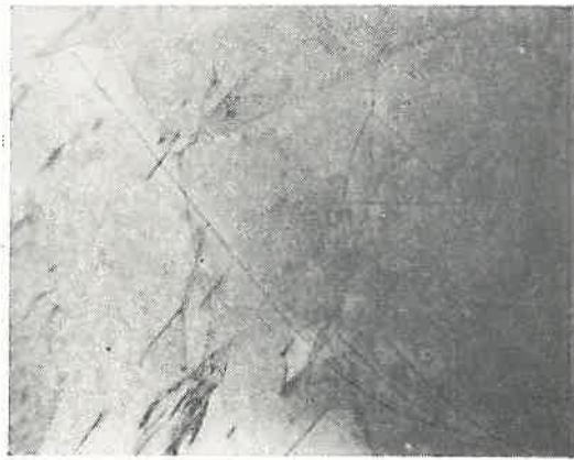
Fig. 3. Long dislocations spreading over the plane (1\bar{1}1) of the secondary slip system, most often observed for samples deformed at high temperatures running through the concentration of short dislocation lines belonging to the primary system
